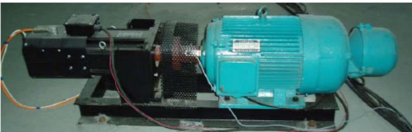
**Fig. 3.** Double-fed generating experiment platform
