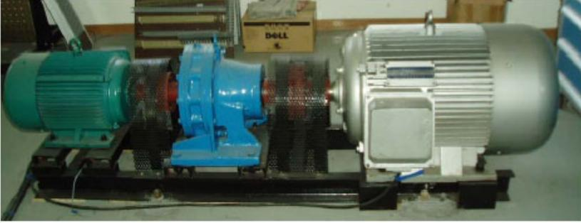
**Fig. 4.** Low-speed permanent magnetic synchronous experiment system
