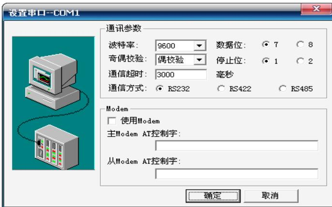
Fig. 6. Communication parameters setting of the Kingview software
