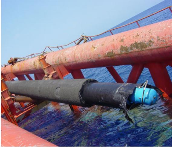
**Fig. 3.** The ruptured pipe
