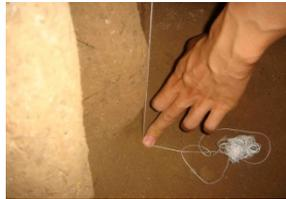
**Fig. 9.** The shear deformation of wheat-lime pile
