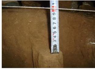
**Fig. 11.** The fracture position of fly ash-lime pile
